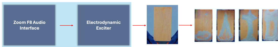
(b) Step 2: From left to right: Illustrative diagram of the measurement chain for the identification of the ODS through Chladni patterns tests.
