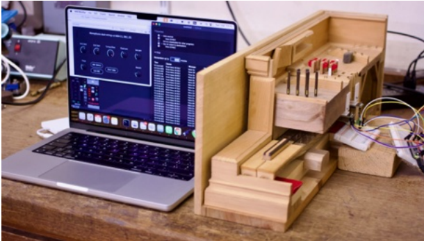
Figure 7: The prototype setup, showing the three-key harpsichord model connected to a 2023 MacBook Pro. The prototype VST is visible, along with a list of triggered MIDI messages.
