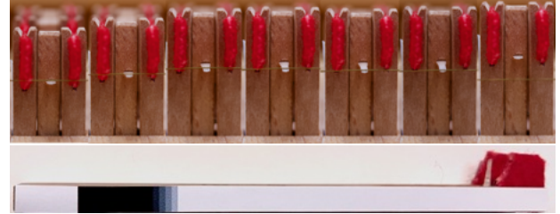
Figure 4: (Top): Snapshots of the plectrum-string interaction during a pluck. Note how the plectrum initially pushes the string but is eventually pushed back by the string before release. (Bottom): side view of a jack showcasing the colour gradient in the reflecting sticker used by the optical sensing mechanism.
