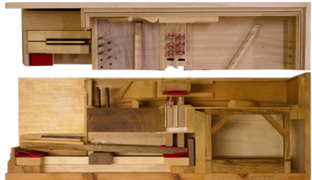
Figure 1: Top and side views of the three-key model built to prototype harpsichord key mechanisms and sensing system.
