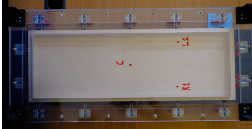
Fig. 4.1 Schematic representation of the measurement setup. The red dots L1 and C indicate the excitation points, namely locations for either the impact hammer hits or the contact point for the exciters while performing the validation measurements, while R1 indicates the position of the accelerometer.
