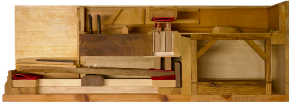
Figure 2.9: Three-key model harpsichord mechanism.
