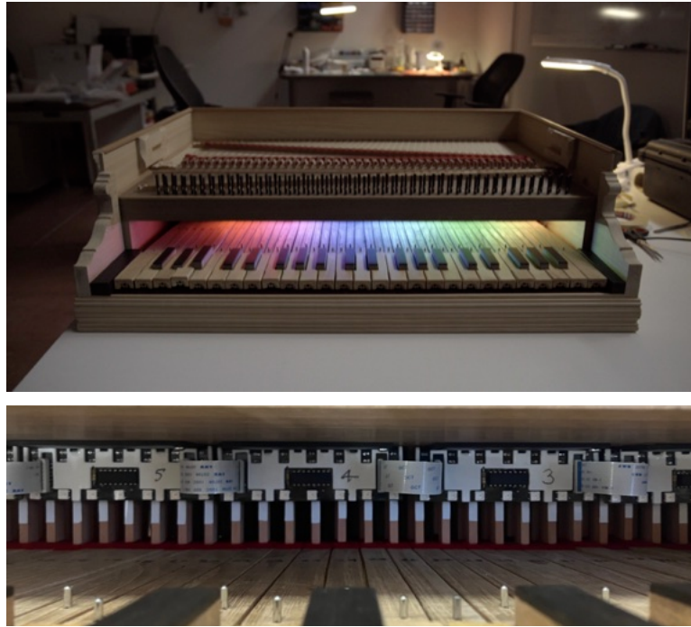
Figure 2.25: Mark II : overall view (top) and front-register sensor boards behind the nameplate (bottom).
