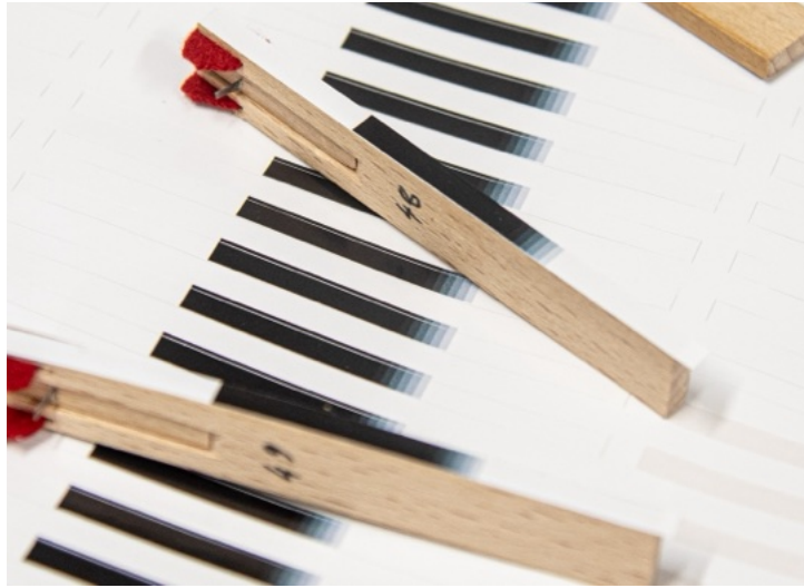
Figure 2.6: Gradient stickers applied to the jack body to provide a concealed optical target.
