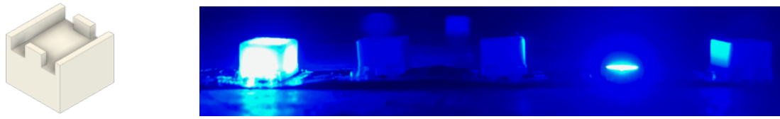
Figure 4.7: Demonstration of light diffusion applied to the RGB LEDs. If mounted horizontally and flush to the wristplank, the source of the light would be difficult to locate, reducing its value as a calibration indicator. Right: example of a bare LED and an LED with a diffuser attached. Left: CAD model of the light diffuser.
